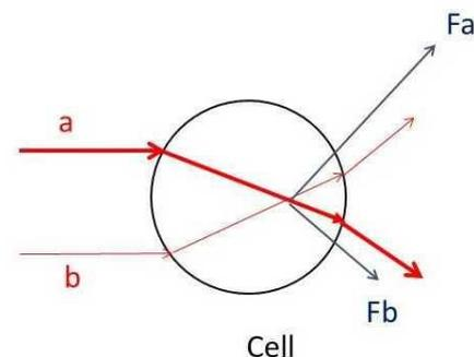
Fig. 1 Forces in an optical tweezer system. Photons a (from the center of a focused laser beam) and photons b (from a peripheral part of the laser beam) are deflected by a transparent particle, e.g. cell. If the number of photons b is smaller than that of photons a, the sum of repulsive forces  $F_a$  and  $F_b$  is directed towards the focus of the laser beam.
