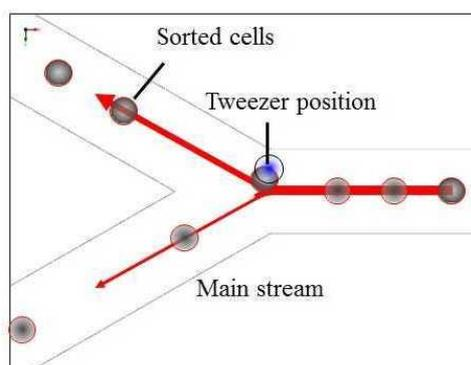
Fig. 2 Rapid cell sorting using a Nd:YAG laser at 1064 nm. Cells are deflected from a main stream by the force of an optical tweezer system (in relation to Ref. [49]).
