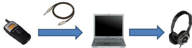
Figure 2. Data acquisition setup for sounds produced by faulty fuel-injectors.
